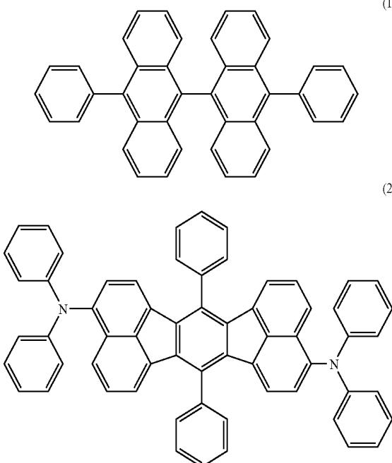
For the blue luminescent medium film, the materials represented by the above-mentioned formula (1) and the following formula (3) were deposited at a ratio of (1) to (3) of 35 to 0.8 in a thickness of 35 nm.
